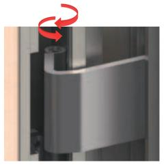
screw positioned on the upper part of the hinges; unscrewing and screwing them with an 6 mm Allen wrench it is possible to correct any height misalignment.
