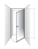
H Max = 2700 mm H1 Door = H - 40 mm L Space max = 1200 mm L 1 Door = L - 66 mm
